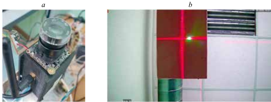
Fig. 6. Laser spot detection system: camera (a); image captured by the camera (b)
