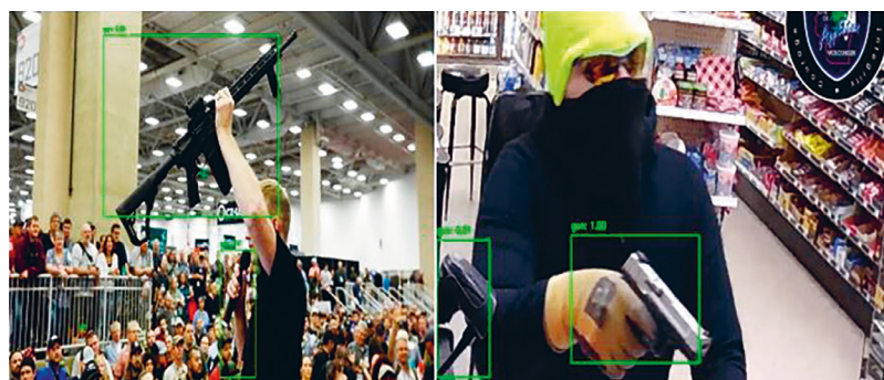
Fig. 12. Misdetections: False positives
