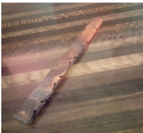
Fig. 6. Designed waveguide with semicircular slots in broad wall
