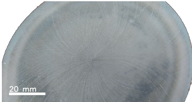
Fig. 4. Machined part after proper tool alignment — protrusion successfully removed
