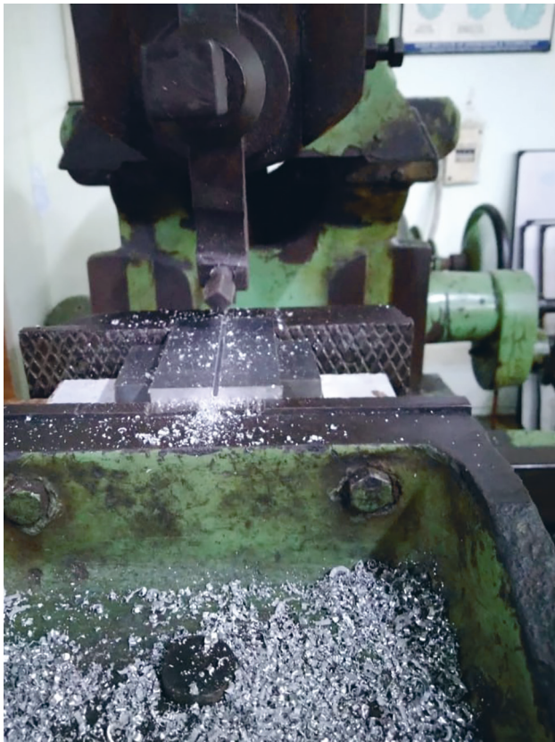
Fig. 5. Grooving on the sample
