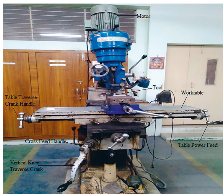
Fig. 7. FSP set-up machine
